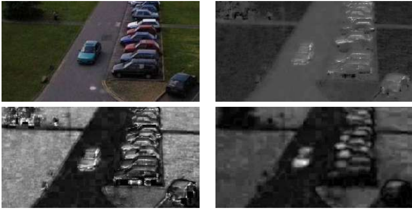
Fig. 28.1. Examples of chromatic components. Lexicographically ordered - Image from the PETS2001 dataset, it's normalised blue component b , normalised saturation (cylindrical HSV), IHLS saturation.
